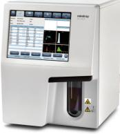
Tri-angle laser scatter + focused flow + chemical dye, creating the possibility for a better 5-part WBC differentiation even on samples with high Eosinophil.
