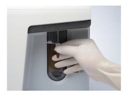
Running capillary blood through the sample probe directly is more convenient for the users in children's hospitals, etc. For Prediluted mode, BC-5000 has higher dilution ratio than other 5-part hematology analyzers, thus it brings a better mixing effect.
