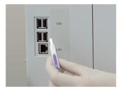
4 USB ports are located on the instrument's left side. They permit BC-5000 users to transmit data conveniently and connect with printers, keyboard, mouse, barcode scanner, etc.
